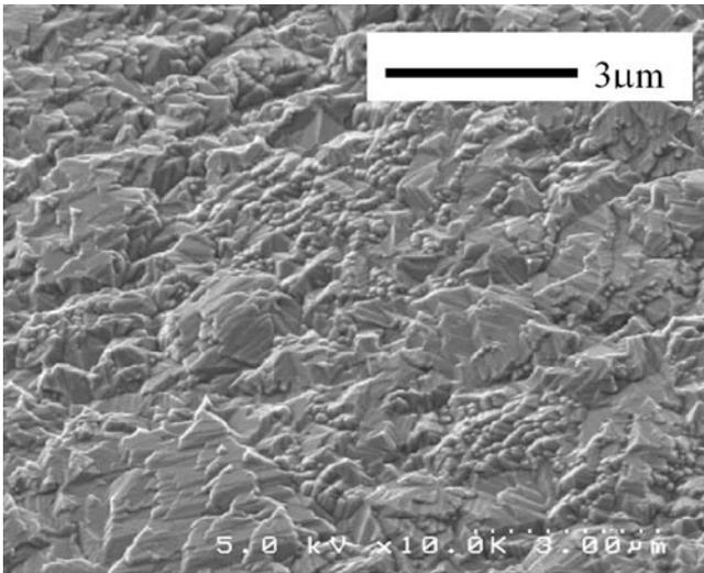
Figure 3—Surface morphology of electroplated copper etched with AES at 40°C by spraying for 5 min.
