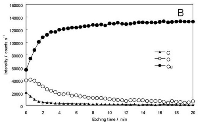
Figure 4—Surface analysis by Auger electron spectrometry: (a) as plated; (b) immersed in AES for 10 min.
