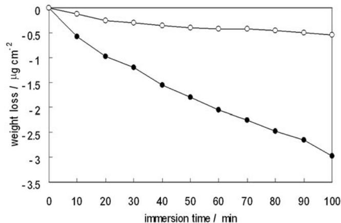
Figure 1—Weight loss of electrolytically copper plated substrate immersed in AES and HCl solution: • - AES, pH 2.2; ○ - HCl solution, pH 2.2.
