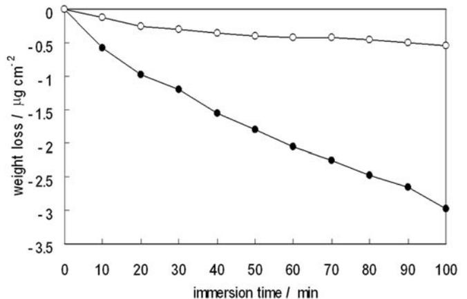
Figure 1—Weight loss of electrolytically copper plated substrate immersed in AES and HCl solution: • - AES, pH 2.2; ○ - HCl solution, pH 2.2.
