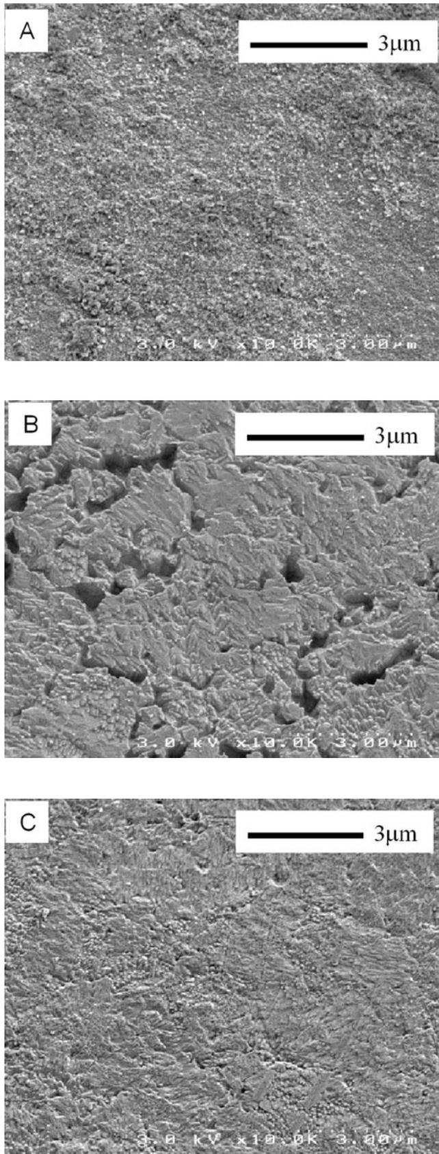
Figure 2—Surface morphology of electrolytically plated copper: (a) as plated; (b) immersed in AES for 10 min; (c) immersed in hydrochloric acid solution for 10 min.
